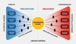
Plant operators identify potential MUEs or "Top Events"—like fires and explosions—each one of these Top Events forms the centre of a bow tie (see diagram above). All plausible accident scenarios that could exist around each MUE are considered and then critical controls that would prevent the Top Event are identified.
