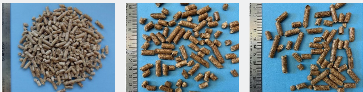
Figure 8 - Wood pellets made from pre-pelletizer feedstocks from left to right: 50% white birch and 50% conifer sawdust; 40% spring and summer birch and 60% conifer sawdust; and 50% spring and summer birch and 50% conifer sawdust.
