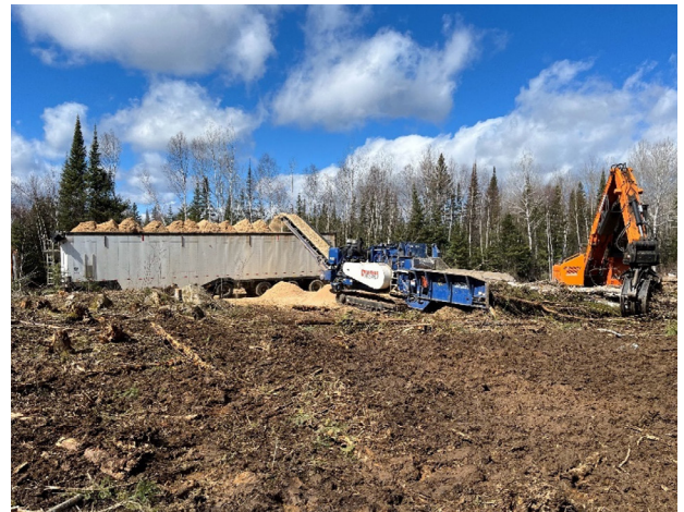
Figure 3 – Forest residue grinding using Peterson 4710B
