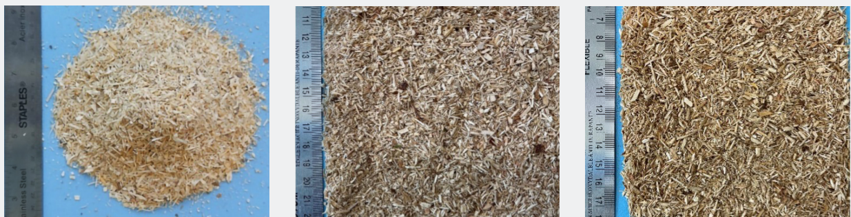
Figure 7 - Pre-pelletizer feedstocks from left to right: 50% white birch and 50% conifer sawdust; 40% spring and summer birch and 60% conifer sawdust; and 50% spring and summer birch and 50% conifer sawdust.
