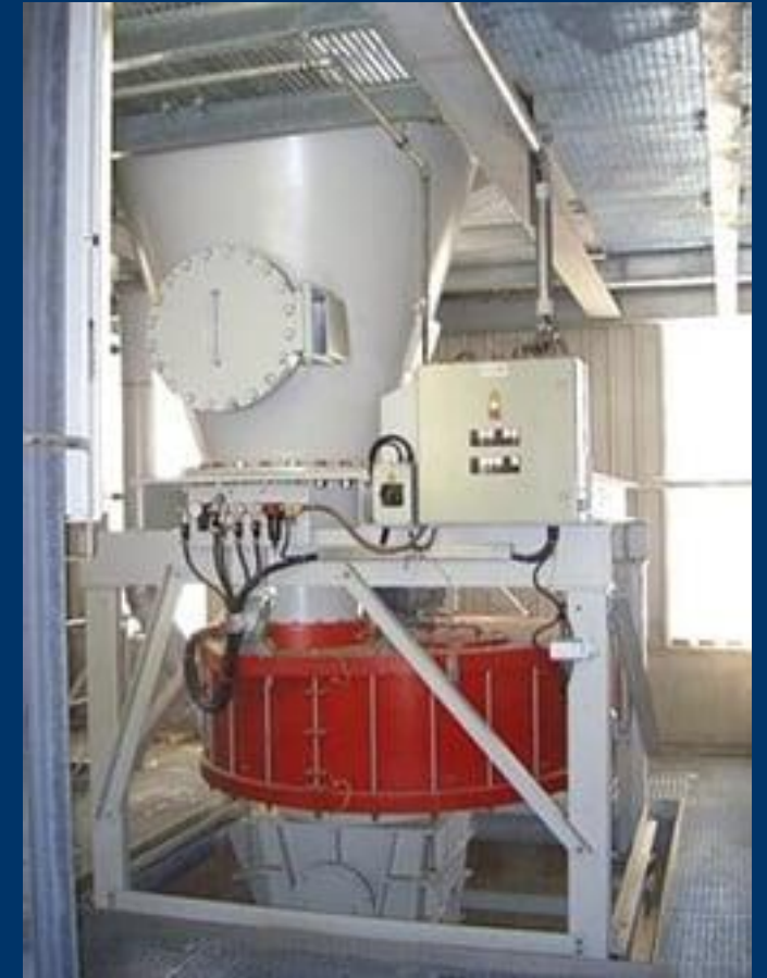
Valmet's wood powder firing solution for lime kilns
