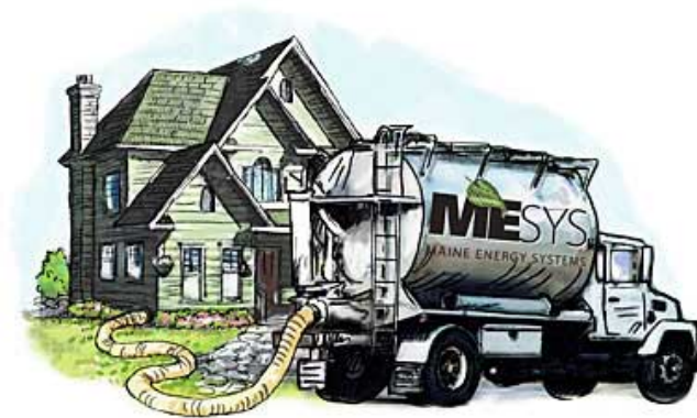
Figure 3: Pneumatic delivery of loose, bulk pellets
