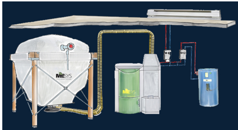
Figure 2: A basic hydronic system with pellet boiler, pellet storage, baseboard radiation, and domestic hot water tank
