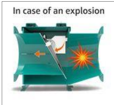
Figure 3-5. During deflagration, valve blade is closed due to pressure wave (Rembe, 2021a) (used with permission)
